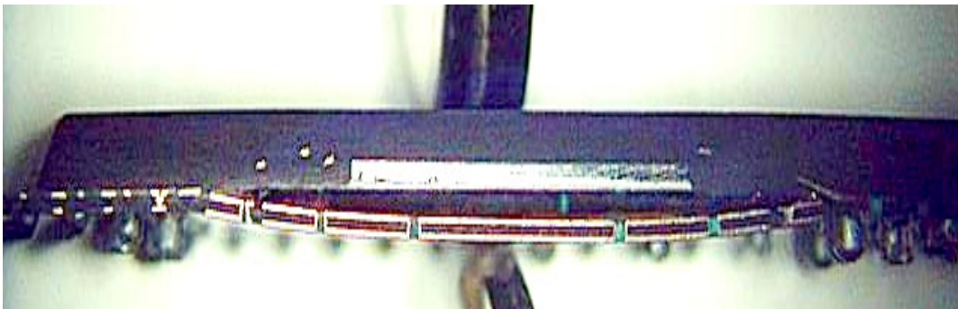
Figure 103. BGA Cross Section Exhibiting Moisture Damage (Popcorning)
