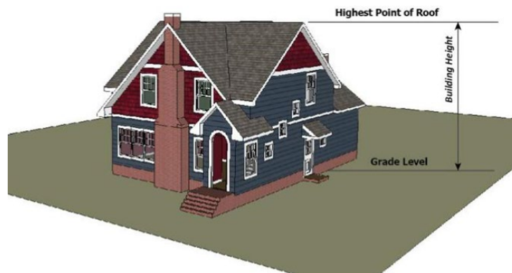
Figure 8-K: Measurement of Building or Structure Height
