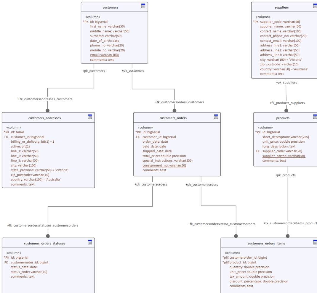
Data modeling diagram with suppressed operation compartment showing tables connected to indicate foreign key relationships.
