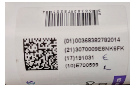
Figure 2. The product’s expiration date and lot number are not clearly denoted or formatted.
